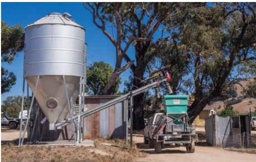
Pig feed stored in a silo on a concrete pad protects the feed from pests and the elements
