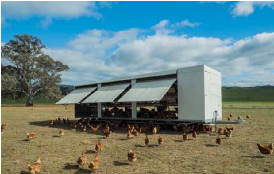
Mobile layer chicken caravan with a 1,000 bird capacity
