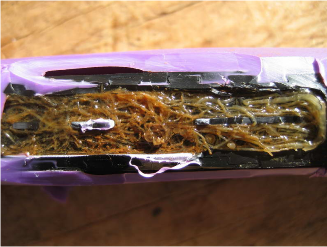
Figure 3. Root penetration into emitters can be an issue for almond producers, particularly in a low water supply situation (Photo: Peter Henry)
