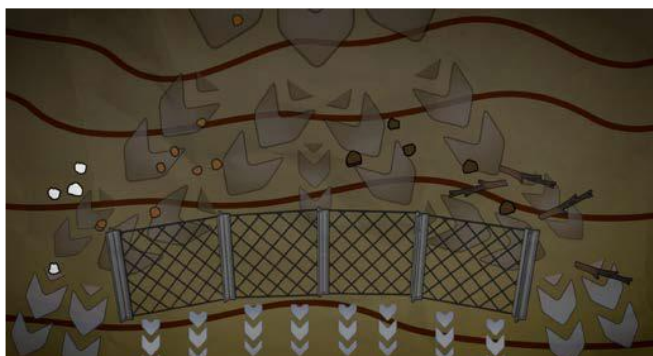
Ensure that the fence line curves downwards at each end so water slows and goes around the fence.
