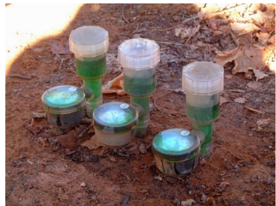
Figure 1. A standard set of tensiometers installed at 30, 60 and 90 cm depth (Image: Jeremy Giddings)
