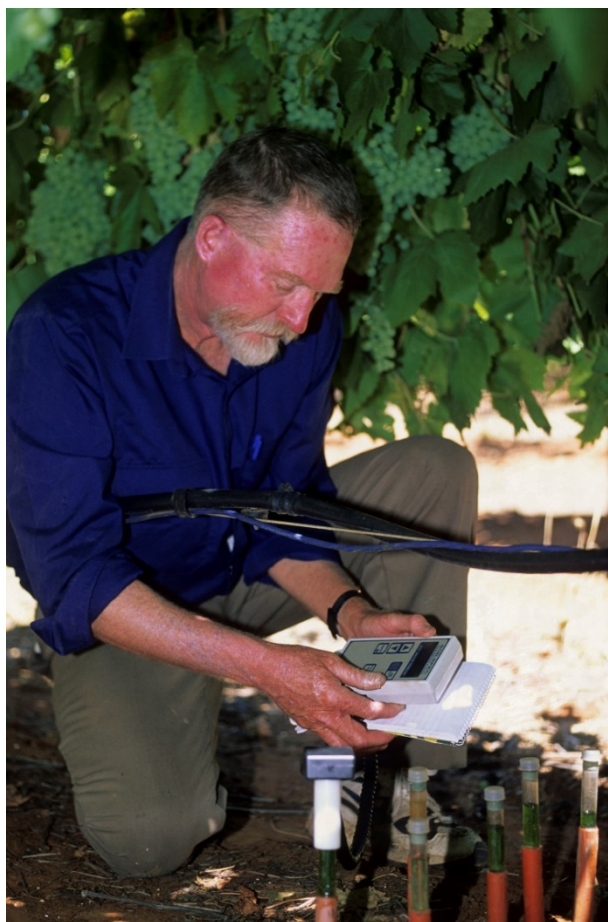
Figure 2. Portable needle type tensiometers (Image: NSW DPI)
